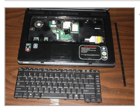
Remove the keyboard completely from the laptop.
