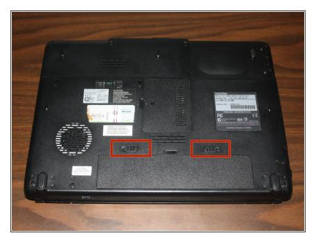
Locate the two sliding battery locks on the underside of the laptop.
