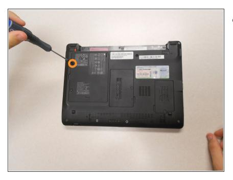
Remove the two screws on the cover with the specified screwdriver.
