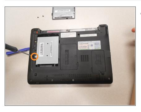
Remove the one screw holding the hard drive in place with the same screw driver.
