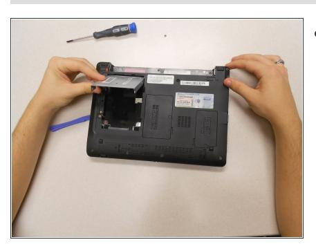
Slide the hard drive up and remove it from the laptop.
