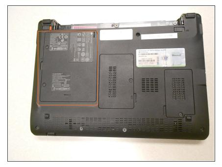
The hard drive is located on the bottom of the laptop on the left hand side.
