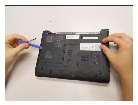
Lift off the cover with the plastic opener.
