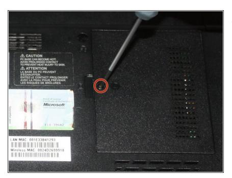
Use a phillips head #0 screwdriver to remove the screw located on the RAM cover.
