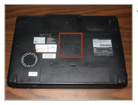
• Locate the RAM cover on the underside of the laptop.
