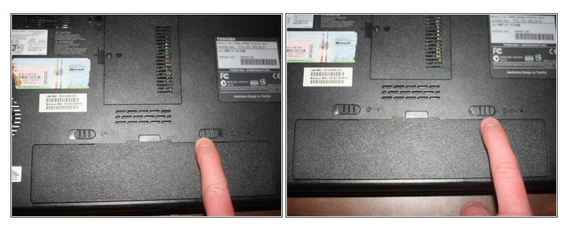
• Locate the right battery lock and slide it to the right.
