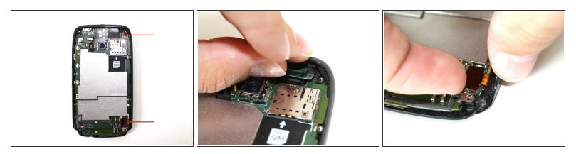
• Disconnect the 2 ribbon cables connecting the LCD & Digitizer to the motherboard
