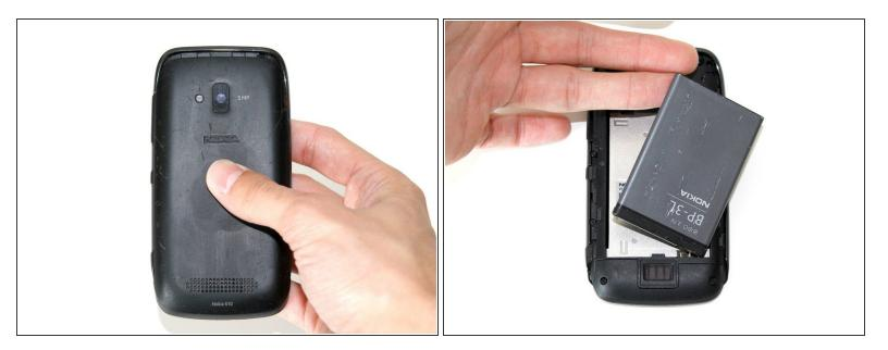
• Slide the back cover off, and remove the battery
