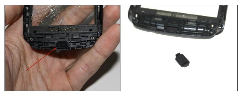
Something very easy to forget - remove the tiny rubber gasket for the microphone, and place it in the new front panel
