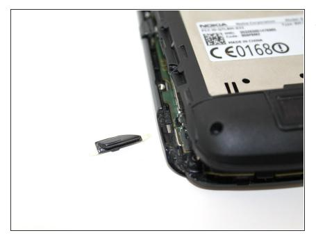
Watch out - the buttons easily fall out; just make sure you don't loose any, a'aight ?!
