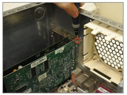
Using a Phillips #0 screwdriver, remove the single 6 mm screw fastening the video card to its mount.
