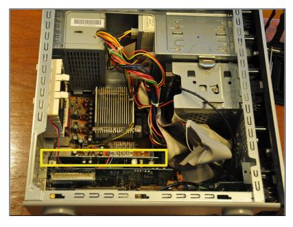
Identify the video card (the green card nearest to the fan casing in the bottom left hand corner of the tower).
