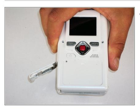
Open battery door. This can be done by gently depressing and sliding the battery down downward.
