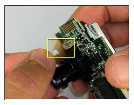
Disconnect the USB port cable from the back side of the circuit board.
