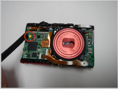
Disconnect the small cable from the yellow port on the motherboard
