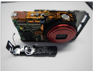
Lift from the back of the camera, angling forward and pull off to remove the power button assembly
