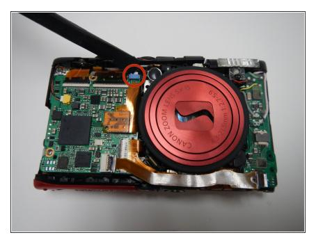
Disconnect the small cable from the blue port on the motherboard
