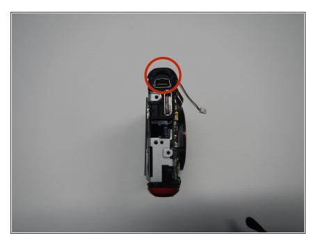
Lift the plastic over the HDMI port on the side of the camera
