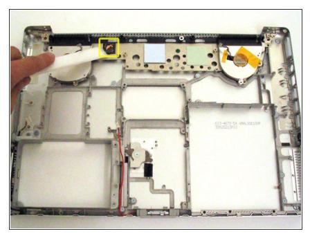
Use a firm plastic edge to scrape the thermal material off the heat sink.
