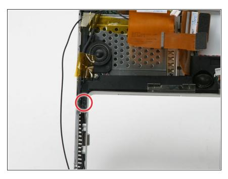
Remove the black Phillips screw on the bottom corner of the left speaker board.
