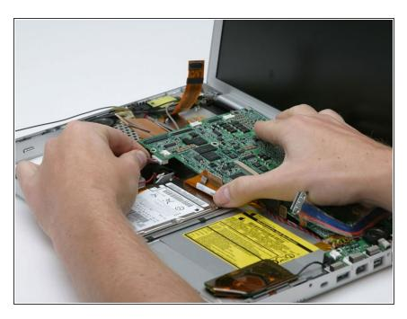
Disconnect the battery cable from the front, left corner of the logic board.
