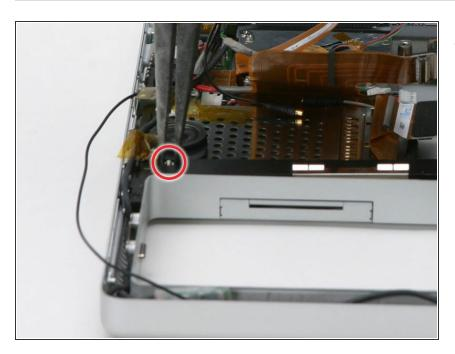
Remove the nut from the screw just in front of the left speaker.
