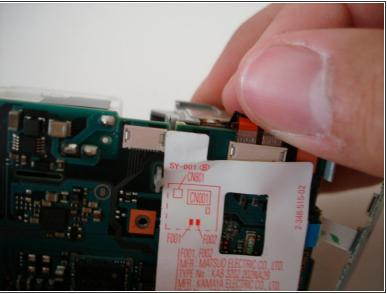
Remove the orange cable connecting the battery terminal to the motherboard.
