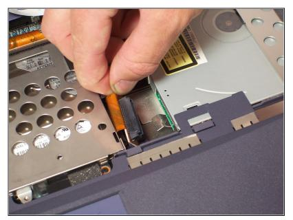
Carefully detach the harness from the CD/DVD drive. Use your fingers if possible, but if not carefully use a pair of <u>tweezers</u> to detach the harness. Take care in not bending any of the pin connections.
