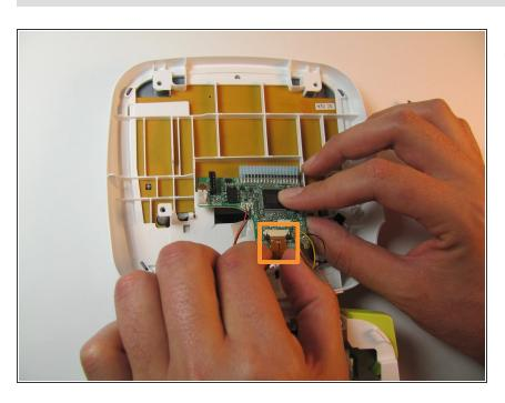
Disconnect the LCD ribbon cable from the circuit board.
