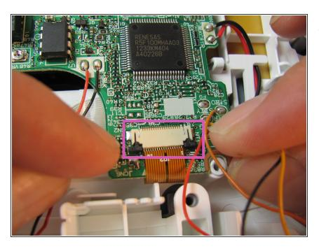
Release the two black clips that hold the LCD cable ribbon in place. To release, pull the clips towards the ribbon.
