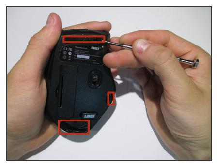
Using a spudger, carefully pry off the stickers to reveal the location of four screws.
