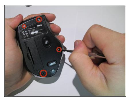
Using your Phillips screwdriver, remove the four screws.
