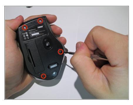
Use a Phillips #00 to remove the 4 screws shown by the red circles in the picture.
