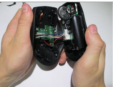
Using a plastic opening tool or spudger, on the center of the mouse, separate the upper and lower board.
