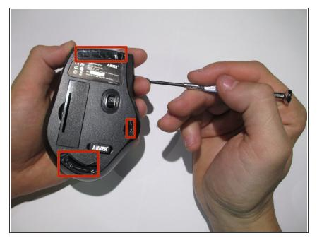
Remove the stickers from the bottom of the mouse to have access to the screws, The stickers are shown in the picture by the red rectangles.
