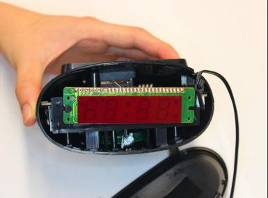
Upon prying the front panel, take care to not puncture the grey shielded connectors for the LCD module.
