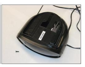
Pry the alarm clock's front panel by applying downward and forward pressure at the two tabs on the edges of the alarm clock. Be careful to not apply too much pressure as the tabs are fragile.
