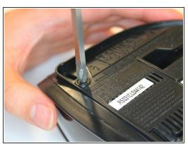
Remove the single screw from the bottom of the alarm clock radio with a Phillips head screwdriver.
