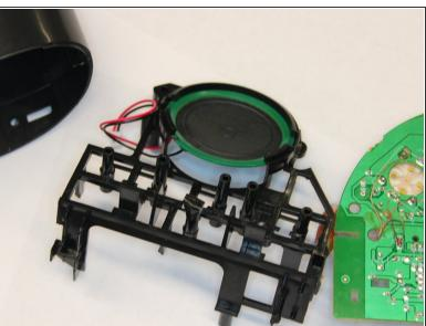
Complete view of the underside of the PCB and the provided speaker.
