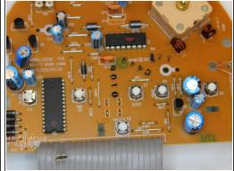
Complete view of the topside of the PCB isolated from the plastic chassis.
