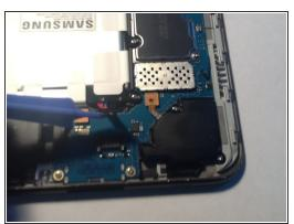
• disconnect the battery by prying from underneath where the wires attach.
