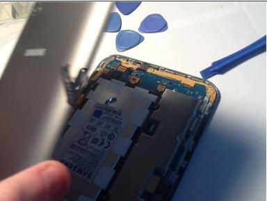
Lift the back plate away from the tab.
