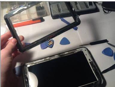
• feed the connector out of the frame.
