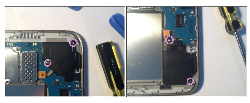
remove the screws holding the speakers in.
