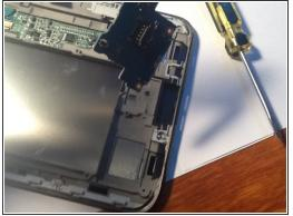
• lift the motherboard out of the device
