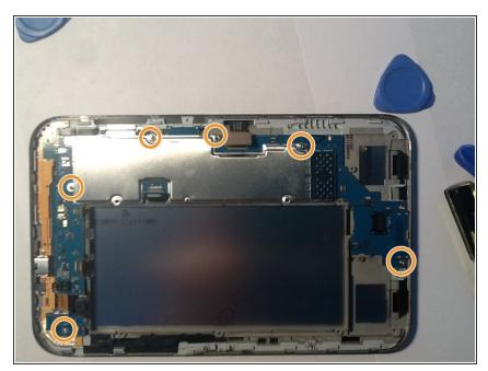
remove the motherboard screws as shown
