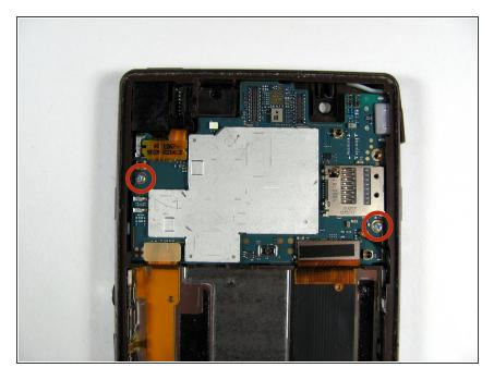
Remove the two 3mm Phillips #000 screws located at the middle left and lower right of motherboard.
