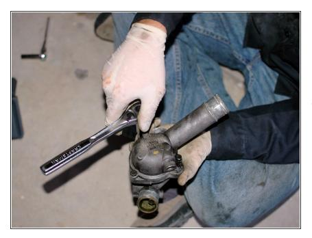
Once the penetrating lubricant has soaked in for a few minutes use your 10mm socket and ratchet to loosen the three bolts that hold the cover on to the thermostat housing.
