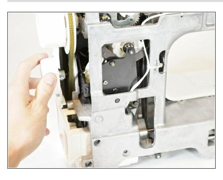
Adjust the knob to gain access to the phillips head screw.
