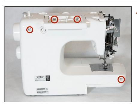
Remove the two 14mm Phillips #2 screws and two 22mm Phillips #2 screws that secure the rear casing.
