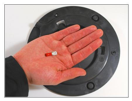
You will need three 16-22 gauge connectors (spaded lugs). The 'gauge' number refers to the wire size the lug connector is designed to fit. These connectors will slip over the contacts on the power coupling.
