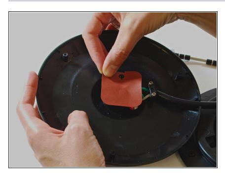
Replace the red square protector on top of the wiring system.
