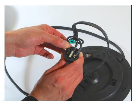
Remove the connectors (spaded lugs) from the kettle's power coupling by gently pulling on each wire.
