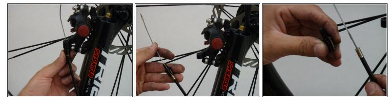
Unscrew the slotted brake cable cap on the rear tire and pull out the cable. Remove the cap from the cable.
