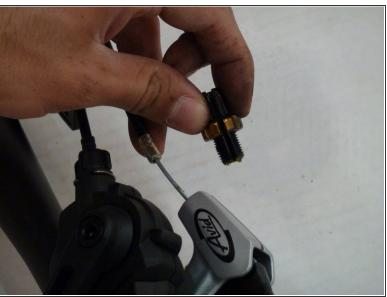
Unscrew the cap next to the brake handle and remove it from the cable.
