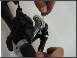
Pull up and out on the cable to remove the barrel nipple (the small cylinder at the end of the cable).
