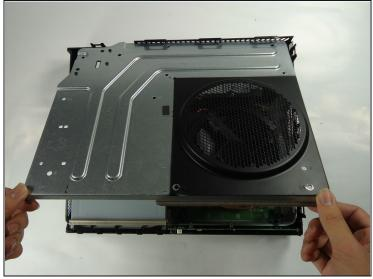
• Remove all eight of the 64.0 mm, T-9 screws labeled C1 through C8 securing the chassis top to the motherboard.
