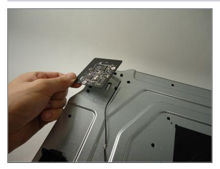
Carefully pull the Wi-Fi board straight up to release it from the chassis. The Wi-Fi board is now free.
