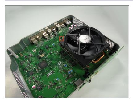
Unplug the wire that connects the fan to the motherboard by gently pulling it up.
