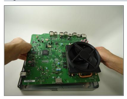
Carefully turn the chassis back over. Grasp the motherboard or the fan and lift the assembly free with the fan and heat sink attached. Set the bottom of the chassis aside.
