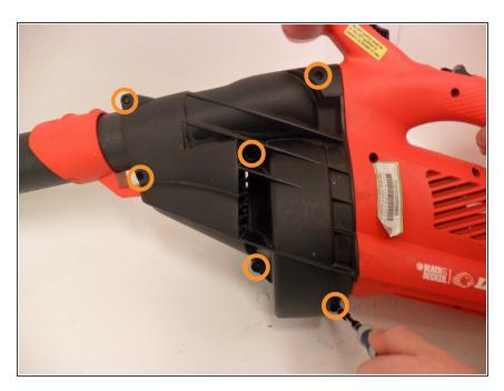
Using a Phillips #2 screwdriver, remove the six 20 mm screws in the black plastic casing (clamshell).
