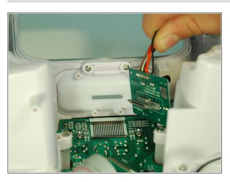
Remove the iPod adapter by sliding it out of the slot.
