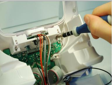
Use a Phillips #1 screwdriver to remove the two 8 mm screws encasing the iPod adapter near the top of the device.
