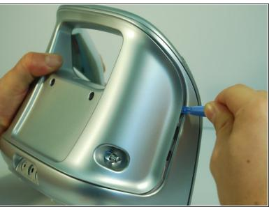
To remove the back panel, use the plastic opening tool and gently work around the outline of the panel. The outline wraps around the sides and can be spotted at the top back of the device.
