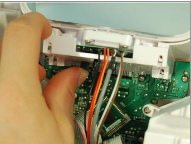
Use moderate force to pry the plastic casing off with your finger while pushing with your thumb against the black, round capacitors.
