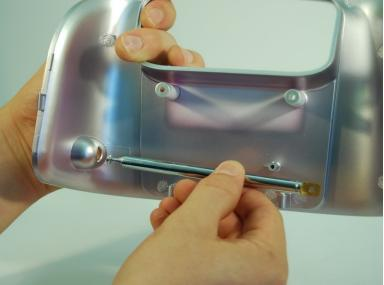
• If desired, the antenna can now be removed by pulling **inwards** and horizontal to the panel bottom.
