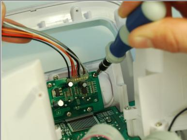
Going back to the small green daughterboard, unscrew the four 6 mm screws with a Phillips #1 screwdriver.
