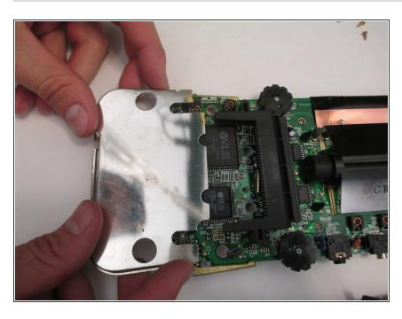
Remove the aluminum back protector to gain access to the C10 capacitor.
