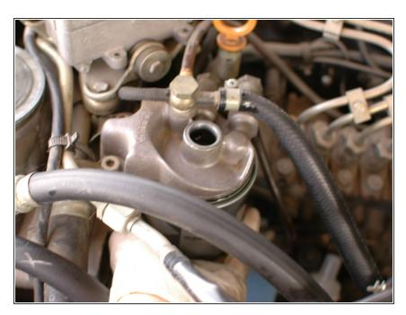
Once the bolt is fully removed, you can now carefully remove the old filter. Be aware that fuel is at the very top of the filter and may spill if you tip it.
