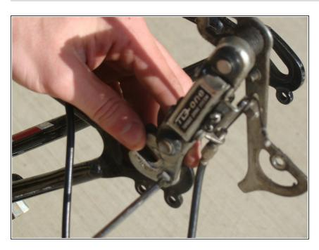
Remove mounting screw that attaches the derailleur to the bicycle frame.
