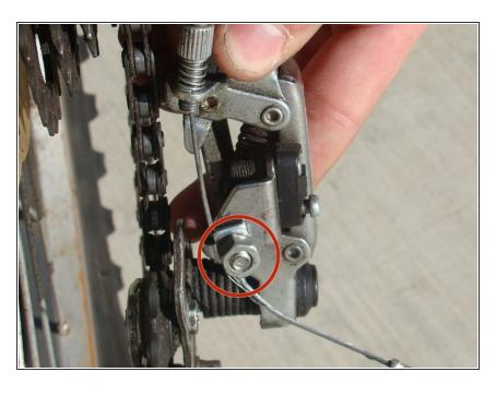
Locate and loosen the hex bolt that clamps the shifting cable.
