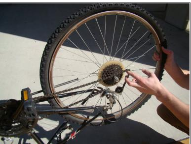
Pull the chain slack and remove the tire.
