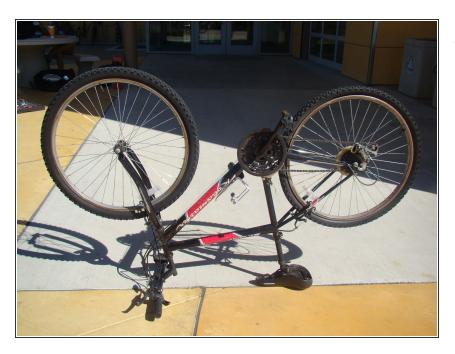
Flip the bicycle upside down so that the bicycle rests on the seat and handlebars. The bike should be able to stay standing on its own.
