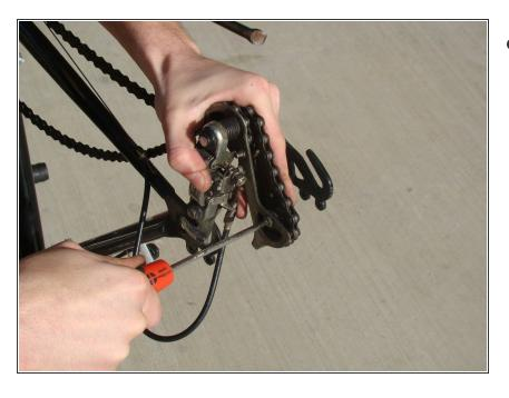
Locate and remove the rear phillips head screw on the sprocket to remove one side of chain guard.
