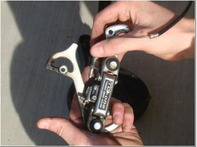
Loosen the shifting cable tension adjustment nut and remove the cable from the derailleur assembly.
