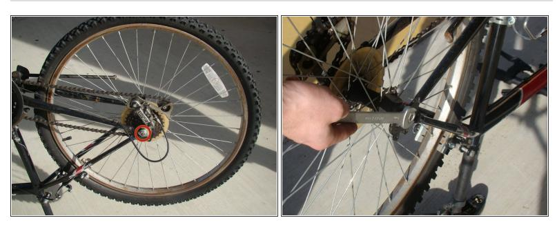
Locate and remove the main axle nuts (both sides) with a 15mm open-end wrench.
