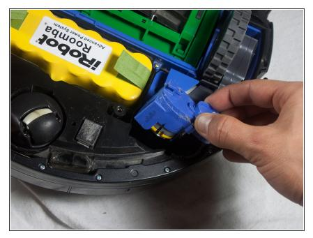
Gently pull on motor assembly to remove.
