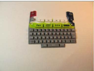
Peel off the rubber keyboard of the device.
