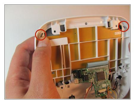
On the top portion of the device there are four grey clips locking the faceplate in place. The two top clips are circled in the image. The two others are located in the other corners of the device.
