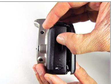
Release the side latch to open the back panel.
