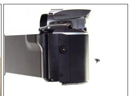
Remove the remote control socket cover.
