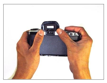
Remove the eyecup from the eyepiece by pushing the eyecup up.
