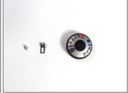
On the top panel, remove the silver 3.8mm Phillips #1 screw right below the command dial.
