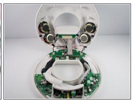
Open the device along its seam.
