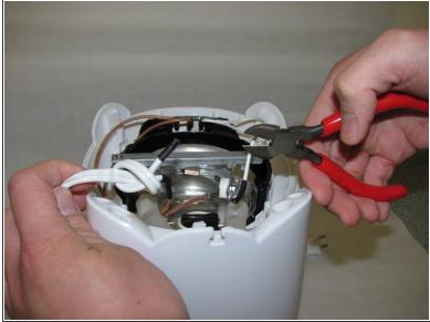
Using a set of wire cutters, cut both leads of the power cord at the heatshrinked area where the leads split.
