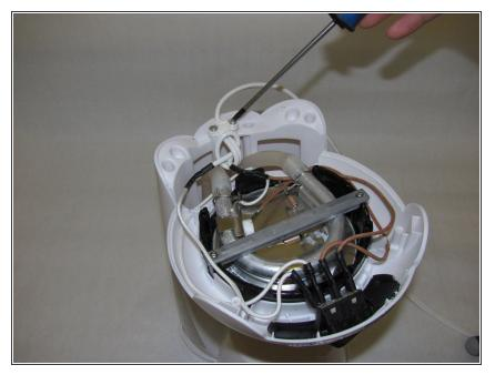
Using a Phillips #1 screwdriver, remove the two 13mm Phillips screws that are securing the wire harness.
