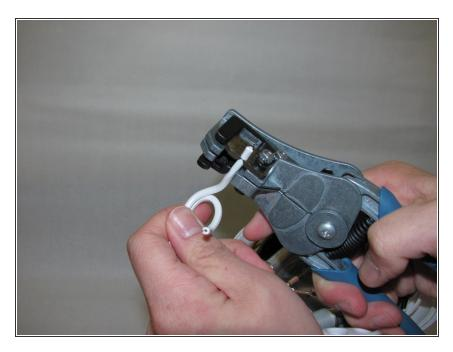
Using a 14-16 AWG wire stripper, strip the leads on the replacement power cord.
