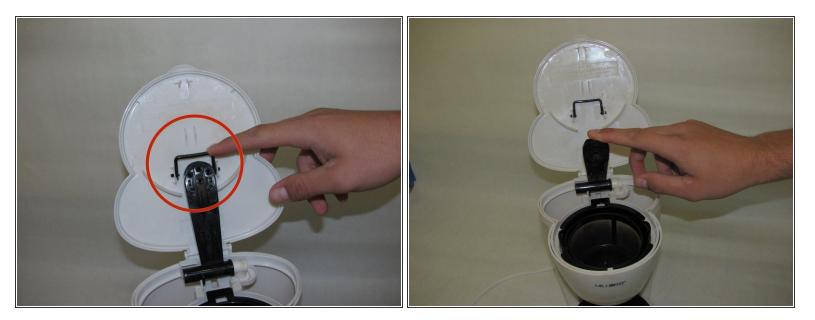
Orient the retaining bracket upwards (away from the main body of unit).
