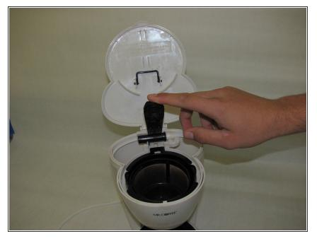
• With the retaining clip in its released position, pull the spout down towards the filter basket.
