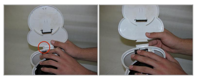
• Carefully detach the dust cover by disengaging the locking pins, starting at one side.
