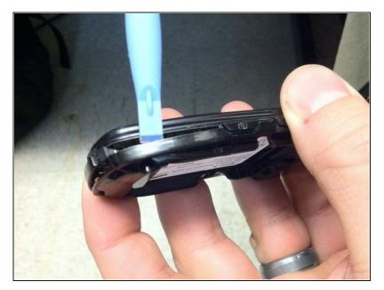
• Using spudger, pry off back cover starting at the bottom corners and moving around the perimeter towards the hinge. Disengaging the clips near the hinge may require some force.
