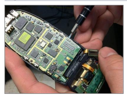
• Using flathead screwdriver, lift motherboard away and remove from phone.
