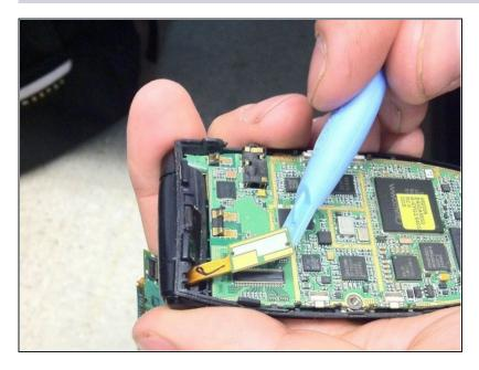
• Using spudger, disconnect electrical connector near the hinge.
