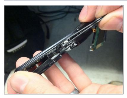
Using <u>tweezers</u>, carefully remove buttons from both sides while removing back cover. Note the positions of the buttons. They must be returned to the proper positions.
