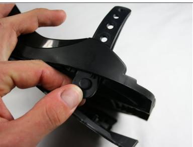
Turn the binding on its side and slide out the toe strap connector.
