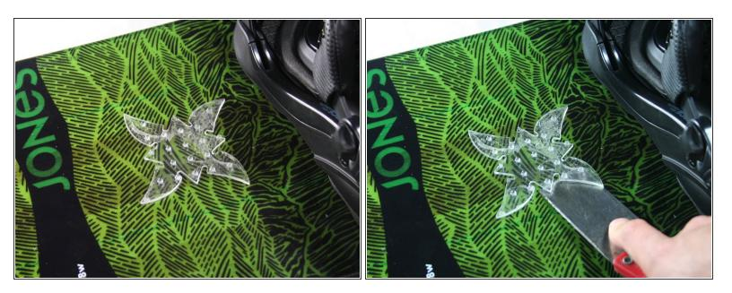
Use a plastic or metal scraper to remove the existing traction pad.
