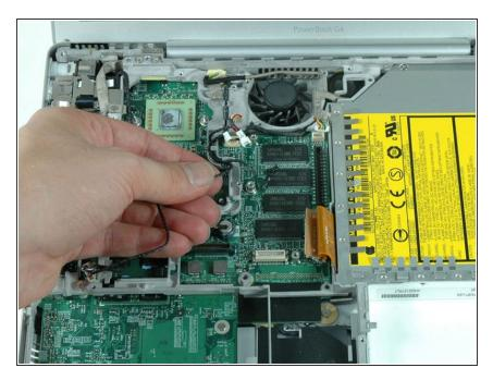
Deroute the microphone cable from its channel in the metal framework.
