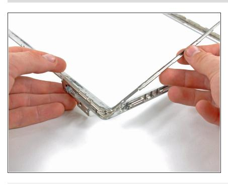
Lift the bar section of the clutch hinge a bit and remove the entire clutch hinge from the front display bezel.
