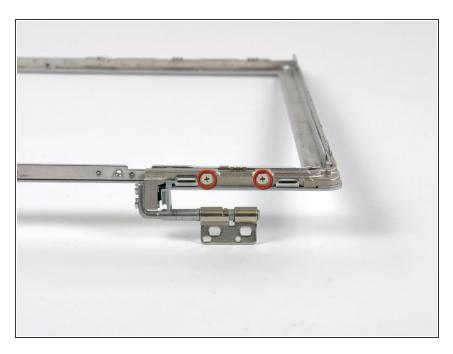
Remove the two 5.5 mm Phillips screws securing the left clutch hinge to the front display bezel.
