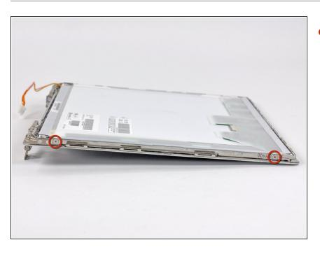
Remove the two 3.0 mm Phillips screws securing the LCD to the left side of the front display bezel.
