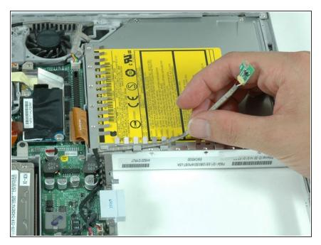
Deroute the cable connecting the hall effect sensor board to the DCto-DC board.
