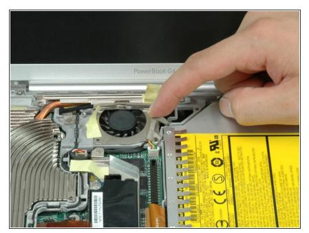
Peel up the Bluetooth cable on the right side of the fan.
