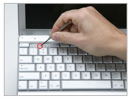
Use your fingernail or a small flathead screwdriver to peel up the gray stickers covering each of the screws.
