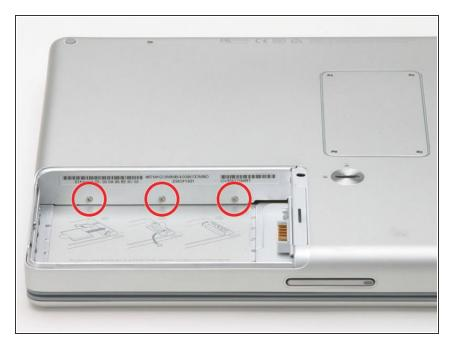
Remove the three 2.5mm Phillips screws from within the battery compartment.
