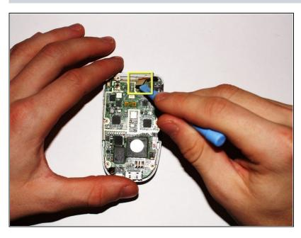
Carefully lift the highlighted connector between the logic board and the screen by using either your fingers or a plastic opening tool as shown in the picture.
