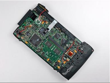
After much (careful) wiggling and prying, the rear case lifts right off the Newton.
