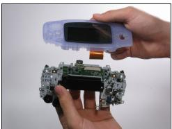
• Using the <u>tweezers</u>, gently pull the ribbon from the logic board.
