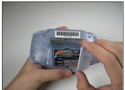
• Take the battery cover off by releasing the locking tab and hinging the cover away. Remove the batteries inside the cover
