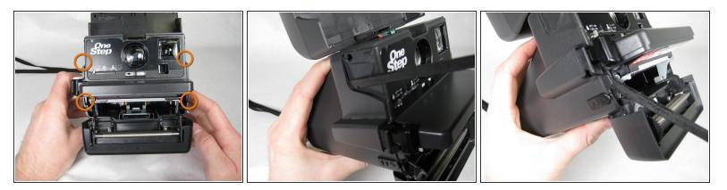
• Insert spudger in between face of camera and sides where the four tabs are located.
