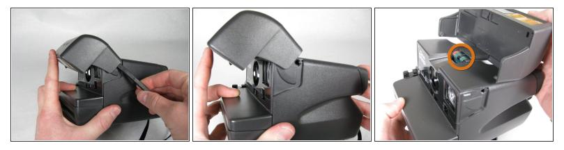
• Separate the flash section of the camera from the main body by unhooking the sides.
