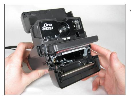
• Open the battery/ cartridge compartment fully.
