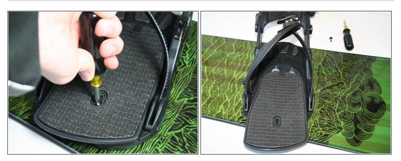
Use a #2 Phillips screwdriver to remove the panhead, 10mm wide, M4 x 12mm screw located in the middle of the foot pad.
