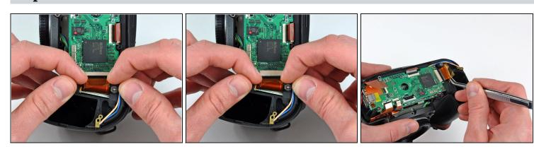
• Use your fingernails to carefully pull the ZIF cable lock away from its socket.
