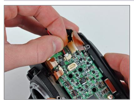
Disconnect the DC-In board connector from the DC/DC board by pulling its connector away from the center of the board.
