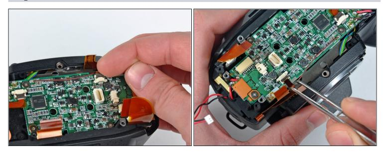
• Use your fingernail to carefully flip up the ZIF cable retaining flap for the ribbon cable socket near the front cover.
