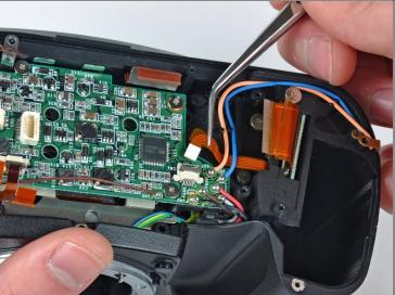
• Use your fingernail to flip up the ZIF cable retaining flap on the socket near the battery opening.
