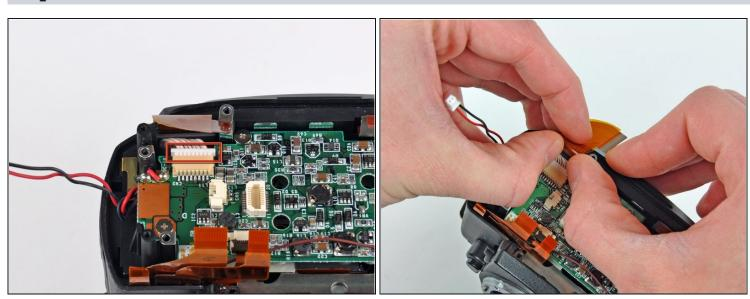
Use your thumbnails to push the CCD connector out of its socket.
