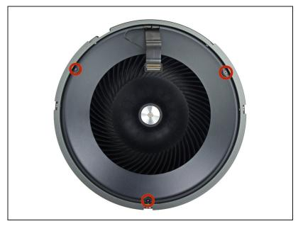
Remove the three 3.7 mm T4 screws securing the fan bezel to the fan assembly.
