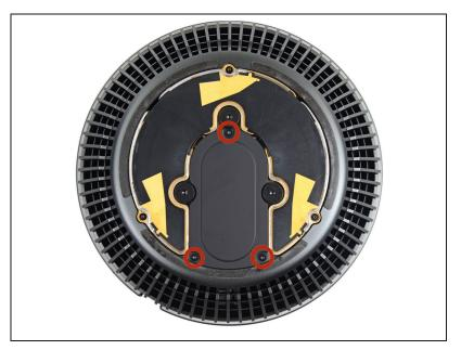
Remove the three 3.7 mm T4 screws securing the metal cover to the AirPort board bay.
