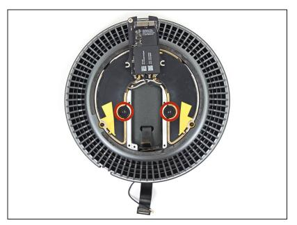
Remove the remaining two 10.4 mm T10 screws securing the fan to the fan assembly.
