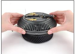
• Lift the fan assembly up from the fan.
