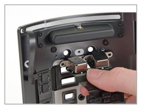
Carefully pull and remove the audio jacks straight away from the IO panel.
