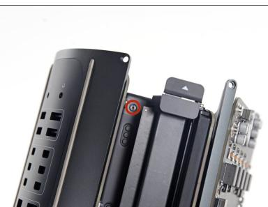
Remove the two 3.6 mm T5 Torx screws from the sides of the power supply cage (one on each side).
