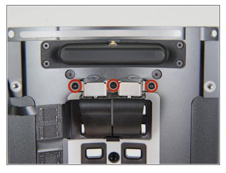
Remove the three 3.7 mm T4 screws securing the audio jacks to the IO panel.
