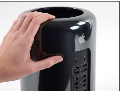
Slide the lock switch to the right, to the unlocked position.
