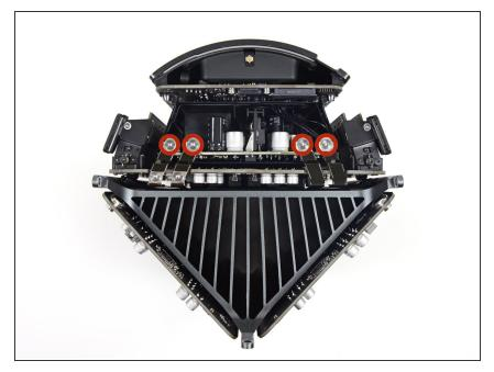
Remove the four 5.5 mm T8 Torx screws securing the power supply assembly to the Mac Pro.
