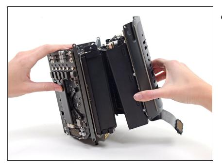
Remove the power supply assembly from the Mac Pro.
