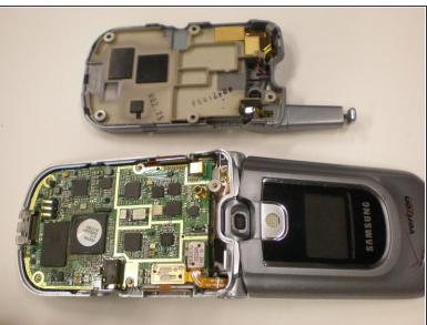
Gently unplug the external speaker wire from the logic board. After the wire is unplugged the back cover should come off easily.
