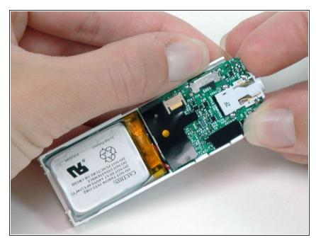
Gently pull back the white plastic framework to free the left edge of the logic board. Pull up on the logic board slightly to prevent the logic board from falling back into place.
