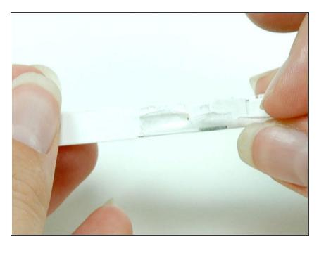
Peel up the translucent tape securing the memory board to the edge of the white plastic framework.
