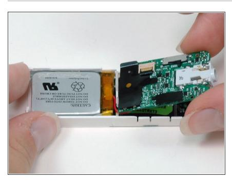
Lift the logic board up to disconnect it from the memory board beneath.
