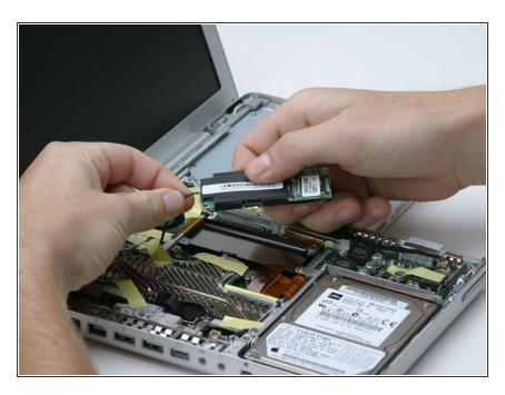
Disconnect the modem cable from the modem.
