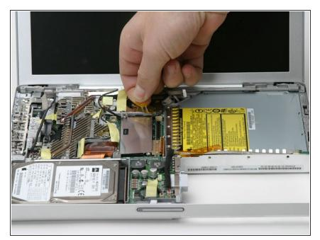
Remove the orange tape on the trackpad side of the fan to free the fan cable.
