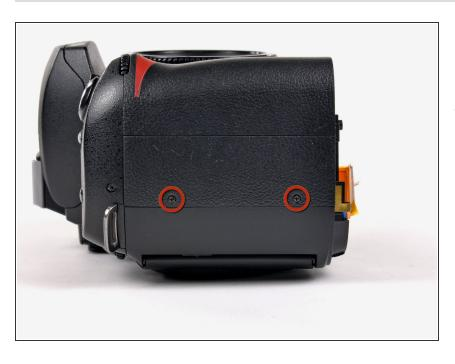
Remove the two Phillips screws securing the grip side of the rear cover to the D70.
