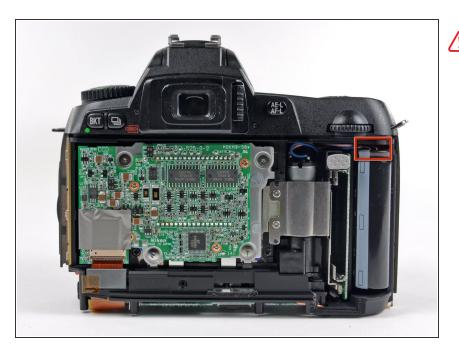
At this point, the capacitor is visible and its exposed contacts are boxed in red. Even though they are recessed, be careful not to touch the contacts to avoid shocking yourself.
