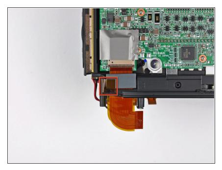
Peel back the piece of tape connecting the iron core around the CCD board ribbon cable to the inner case.
