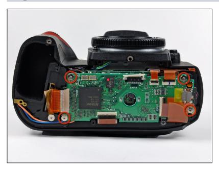
Remove the four 4.3 mm Phillips screws securing the memory compression board to the D70.
