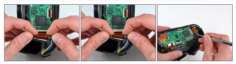
• Use your fingernails to carefully pull the ZIF cable lock away from its socket.
